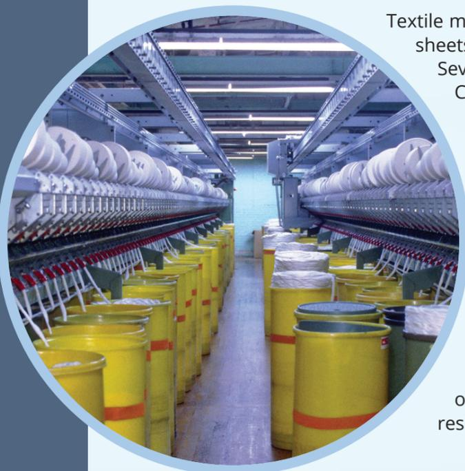
Textile mills spin the cotton fibers into the threads, which are then woven or knitted into clothing, sheets, towels and other cloth items. Textile mills purchase cotton bales based on their classing. Several bales of the same class are blended together to make a consistent group of fibers. Carding machines process more than 100 pounds of cotton per hour into a funnel-shaped device called a trumpet. The trumpet produces a soft, rope-like strand of cotton known as a sliver (pronounced SLY-ver).
